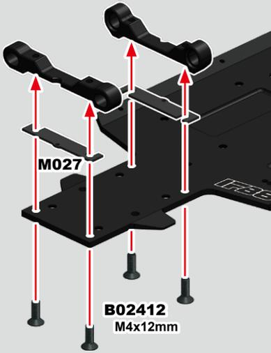
When the spacer is used, we rise the roll center and we decrease the car rolls. If the spacer is used, it's better to use longer screws (M4x12mm flat head screw) instead of M4x10mm.
