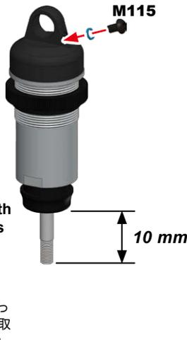
Slowly move the shock shaft up and wipe the excess oil with a rag. While the shaft is in this position place the gasket and M2.5x4mm screw and tighten gently.
