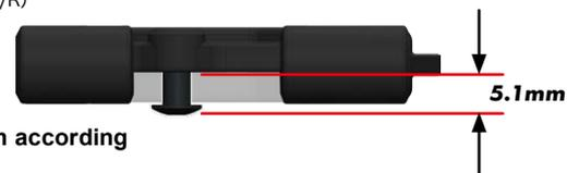
Set the M002 droop screw position according to the setup sheet measurement.
