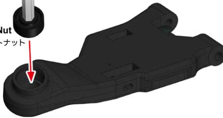
Tighten the M013 ball adjusting nut straight into the front lower arm to create a thread. Then, remove M013 once.
