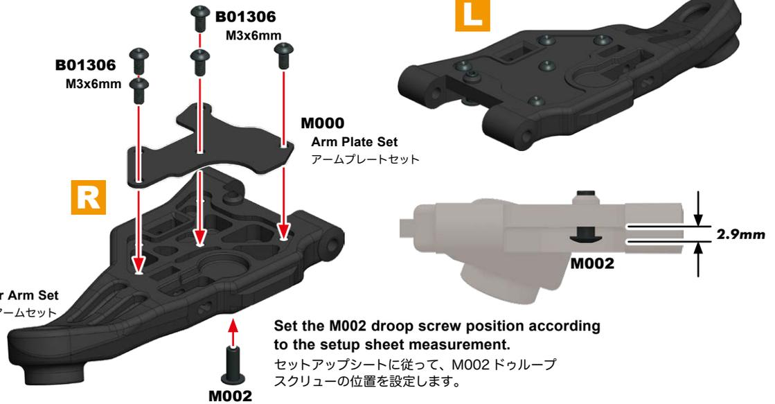
Set the M002 droop screw position according to the setup sheet measurement.
