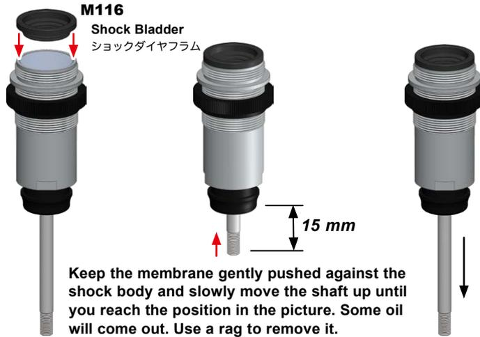
Keep the membrane gently pushed against the shock body and slowly move the shaft up until you reach the position in the picture. Some oil will come out. Use a rag to remove it.
