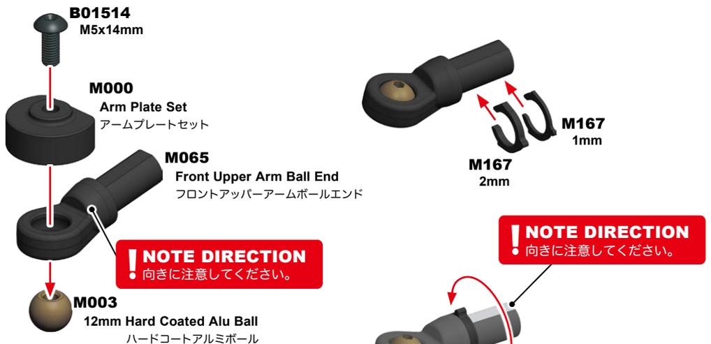
Assemble the M065 upper front arm ball end and M003 12mm ball utilizing the M000 12mm ball jig and B01512 M5x14mm button head screw.
