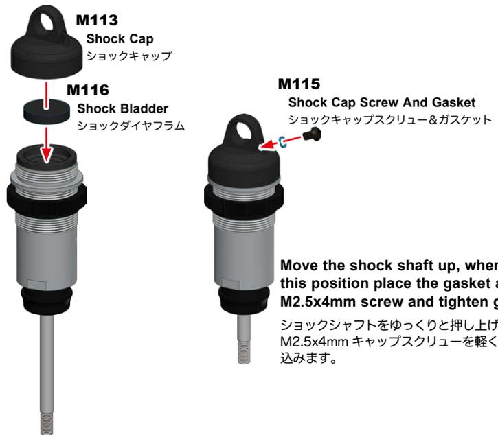
Move the shock shaft up, when in this position place the gasket and M2.5x4mm screw and tighten gently.
