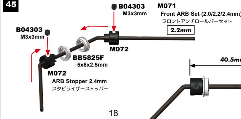
**M072 ARB stopper 2.4mm** can be used to install 2.0, 2.2 and 2.4mm front anti roll bar on your car.
