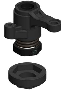
You can use the jig to install the M054 and to adjust the M055 servo saver spring tension. The hex on the jig is 17mm so you can use the same tool you use to tight the wheel nut.
